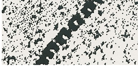
Fig. 6. Caterpillar structure of a monopole track (enlarged \approx 150 times).
